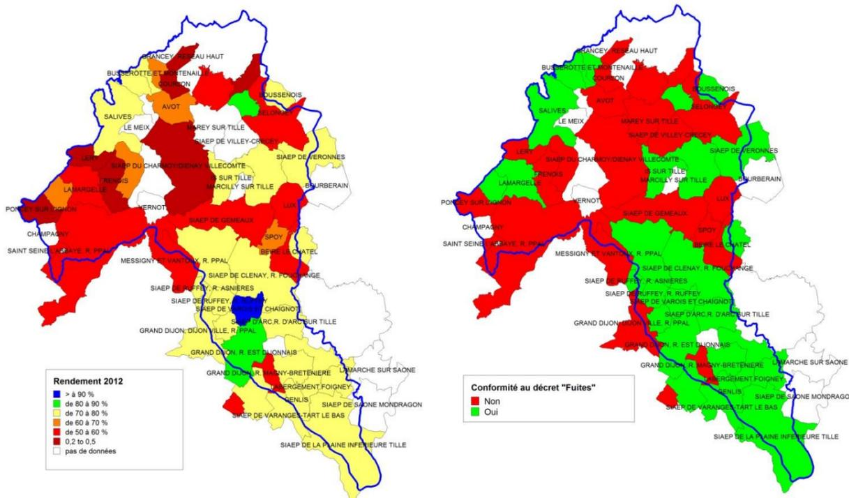
FIGURE 25: RENDEMENT CONNU DES RESEAUX AEP ET CONFORMITE AU DECRET "FUITE" EN 2012<sup>11</sup>
