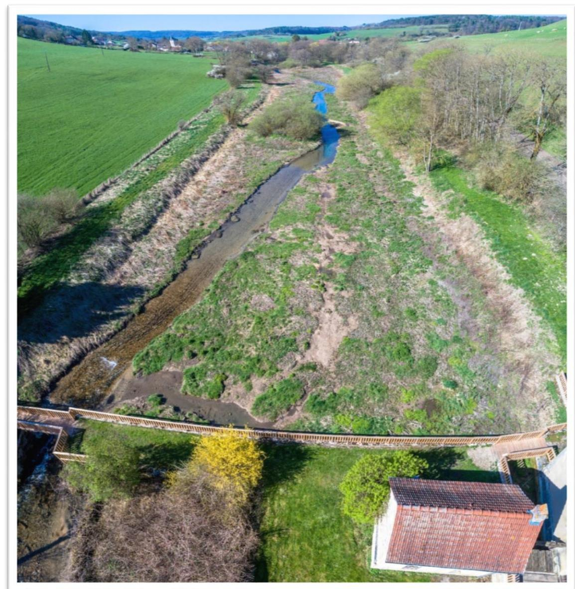
FIGURE 55: L'IGNON RESTAUREE (BAS – APRES TRAVAUX) DANS LA RETENUE (HAUT – AVANT TRAVAUX) DU BARRAGE DU MARTINET DEMANTELE A PELLEREY
